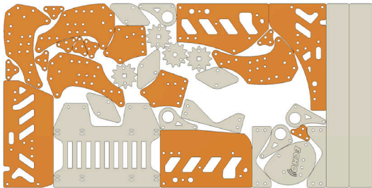
Polycarbonate Used for Drive (highlighted):
