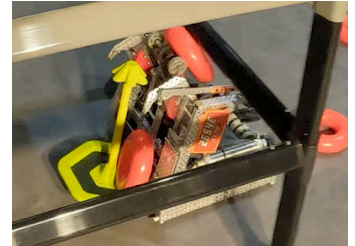
Figure: Robot getting stuck in the center due to rings
